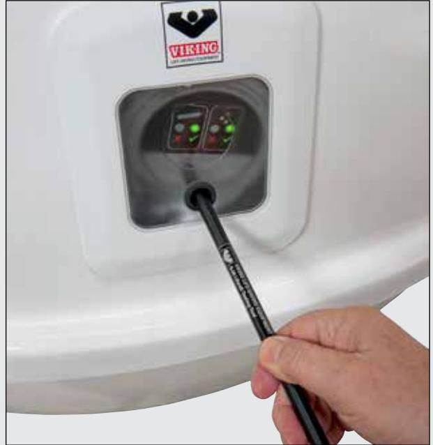
VIKING S30 liferafts feature an extra window at the end of the container to make visual onboard inspection possible.
